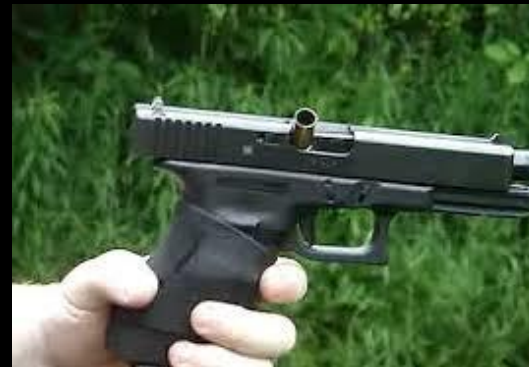
Failure to eject
